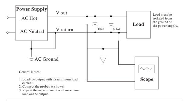
Figure 1. Differential Noise Test Setup
