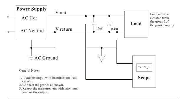
Figure 1. Differential Noise Test Setup
